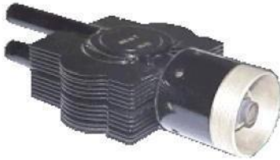
Figure 3.9: Magnetron M 29Г of the old russian Radar “Bar Lock”
