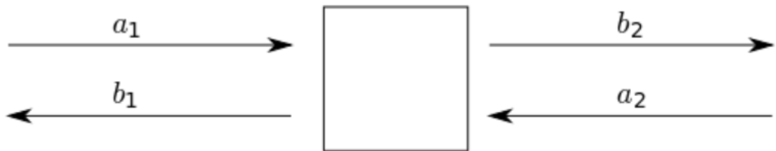
Figure 1.6 Signal Flow in a two port network
